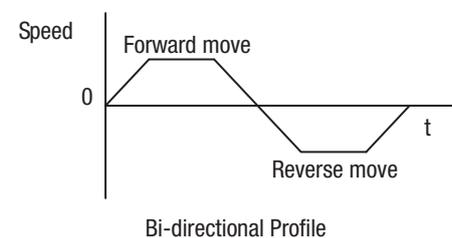
**Note** The MX2 can move loads in both directions. However, it is not designed for use in servo-type applications that use a bipolar velocity signal that determines direction.
