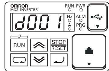
**Output frequency (speed) set** – Resuming keypad operation from the previous table, follow the steps below.
