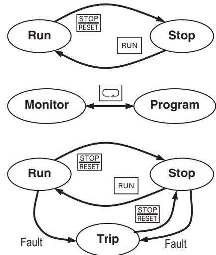
The occurrence of a fault during operation will cause the inverter to enter Trip Mode as shown. An event such as an output overload will cause the inverter to exit the Run Mode and turn OFF its output to the motor. In the Trip Mode, any request to run the motor is ignored. You must clear the error by pressing the Stop/Reset switch. See 6-2 *Monitoring Trip Events, History, & Conditions* on page 273.
