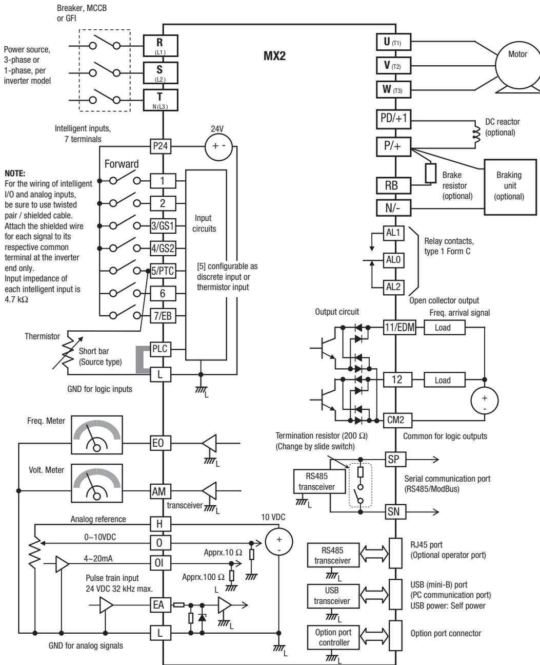
MX2 control wiring quick reference (IP54)
