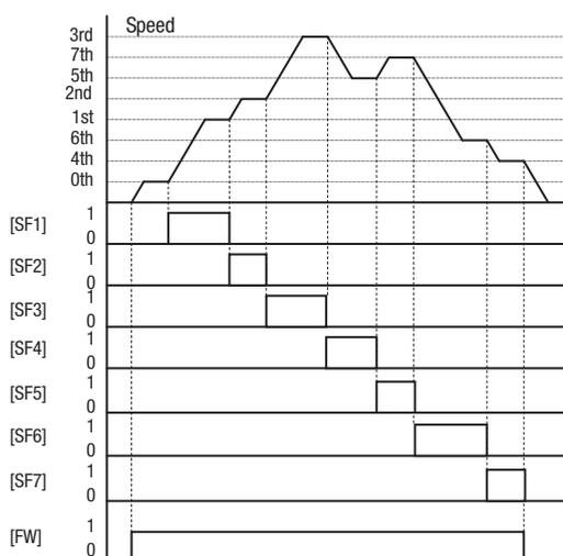
The example with eight speeds in the figure below shows how input switches configured for SF1-SF7 functions can change the motor speed in real time.
