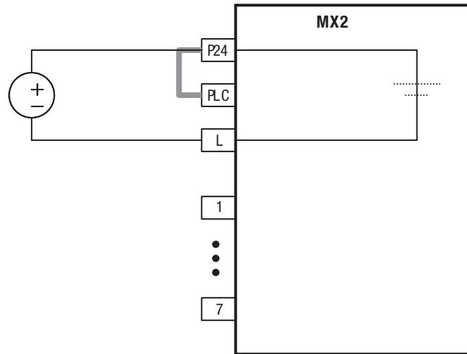
By having ability inverter doesn't block the current flowing into itself when it is not powered. This may cause the closed circuit when two or more inverters are connected to common I/O wiring as shown below to result in unexpected turning the on the input. To avoid this closed circuit, please put the diode (rated: 50 V/0.1 A) in the path as described below.
