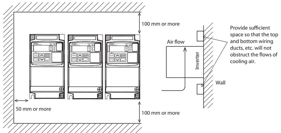
Make sure the ambient temperature remains within the rated range (–10 to 50°C). Take note that if the ambient temperature reaches or exceeds 40°C, the carrier frequency and output current must be derated (check derating tables per each inverter model in *Derating Curves on page 9*). If the Inverter is used in an environment exceeding the allowable operating temperature range, the product life of the Inverter (specifically, the capacitor) will be shortened.
