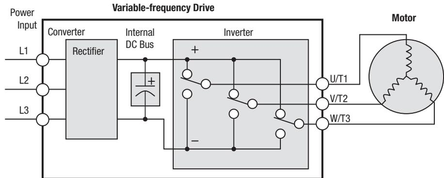
Capacitor life is reduced in higher ambient temperatures, as the graph below demonstrates. Under the condition of average ambient temperature 40°C, 80% load, 24 hours operation, the lifetime is 10 years. Be sure to keep the ambient temperature at acceptable levels, and perform maintenance inspections on the fan, heat sink, and other components. If the inverter is installed on a cabinet, the ambient temperature is the temperature inside the cabinet.
