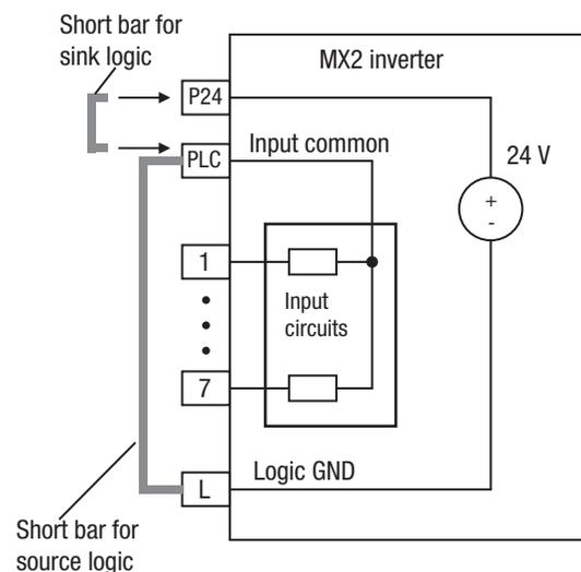
The wiring diagram on the following pages show the four combinations of using sourcing or sinking inputs, and using the internal or an external DC supply.
