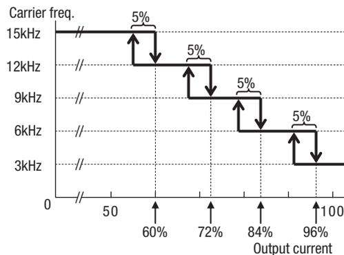
When the output current increases to 60%, 72%, 84%, or 96% of the rated current, this function reduces the carrier frequency to 12, 9, 6, or 3 kHz, respectively. This function restores the original carrier frequency when the output decreases to 5% lower than each reduction start level.
