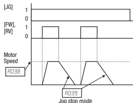
To enable the Run key on the digital operator for jog input, set the value 01 (terminal mode) in A002 (Run command source).
