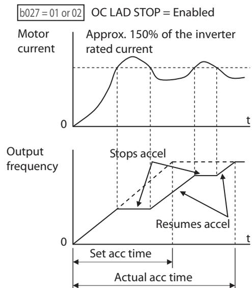
When the Over-current Trip Suppression feature is enabled by b027=01, the inverter stops the acceleration ramp in each case until the motor current level is again less than the threshold value, which is approximately 180% of the rated current of the inverter.
