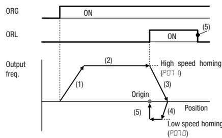
1. The inverter accelerates the motor for the specified ramp time to the high speed homing.
