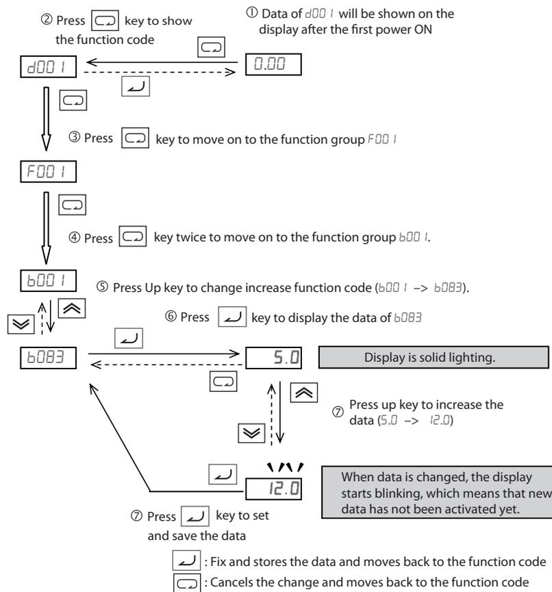
**Note** Function code **bxxx** are for monitor and not possible to change. Function codes **Fxxx** other than **FHHH** are reflected on the performance just after changing the data (before pressing key), and there will be no blinking.
