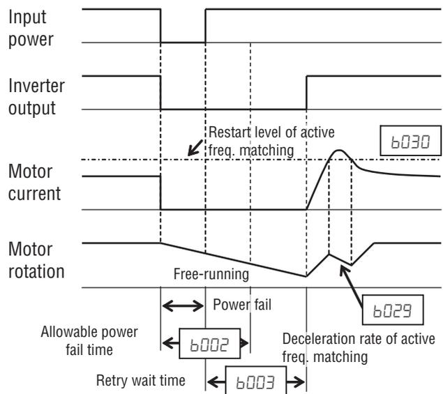
When the motor current is less than **b030**, the inverter increases motor speed toward the set speed. The inverter continues this retry process until the motor speed comes to the previous set speed.
