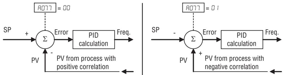
**PID deviation output** - If PID deviation "ε" exceeds the value in **C044**, output signal configured as **D04** (OD) is activated.
