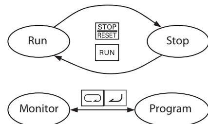
**Note** Some factory automation devices such as PLCs have alternative Run/Program modes; the device is in either one mode or the other. In the Omron inverter, however, Run Mode alternates with Stop Mode, and Program Mode alternates with Monitor Mode. This arrangement lets you program some value while the inverter is operating – providing flexibility for maintenance personnel.
