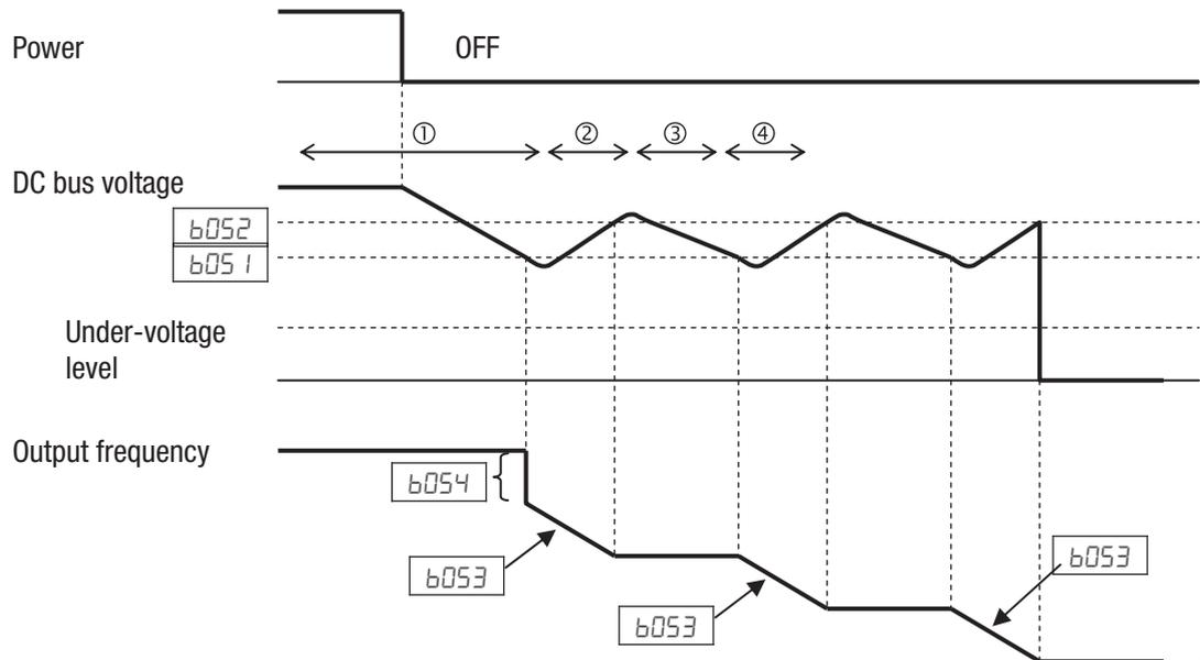
Should power be lost while the inverter is in run mode, this function will have the following effect:
