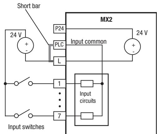
The power to the inverter control part can be supplied externally as shown below. Except driving motor, it is possible read and write the parameters by keypad and via communication even the drive itself is not powered.
