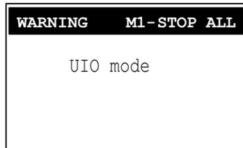
However, when changing to “Unprotected Inverter Operation mode” and a warning occurs, the warning code is displayed in d090 (Warning monitor).
