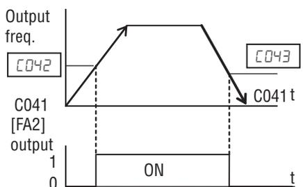
**PID FBV Output** - The Error for the PID loop is the magnitude (absolute value) of the difference between the Set point (desired value) and Process Variable (actual value). The PID output deviation signal [OD] (output terminal function option code 04) indicates when the error magnitude has exceeded a magnitude you define.
