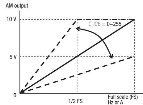
**Note** As mentioned above, first adjust the offset, and then adjust the gain. Otherwise the required performance cannot be obtained because of the parallel movement of the offset adjustment.
