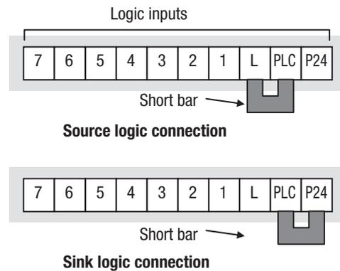
**Caution** Be sure to turn OFF power to the inverter before changing the short circuit bar position. Otherwise, damage to the inverter circuitry may occur.
