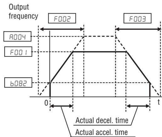
Acceleration 1 and Deceleration 1 are the standard default accel and decel values for the main profile. Accel and decel values for an alternative profile are specified by using parameters *Rx92* through *Rx93*. The operator rotation direction selection (*F004*) determines the direction of rotation as commanded only from the keypad. This setting applies to any motor profile (1st or 2nd) in use at t particular time.
