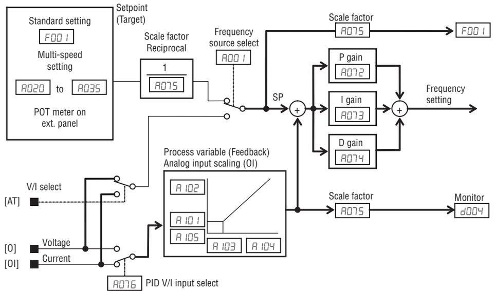
**Caution** Be careful not to turn PID Clear ON and reset the integrator sum when the inverter is in Run Mode (output to motor is ON). Otherwise, this could cause the motor to decelerate rapidly, resulting in a trip.
