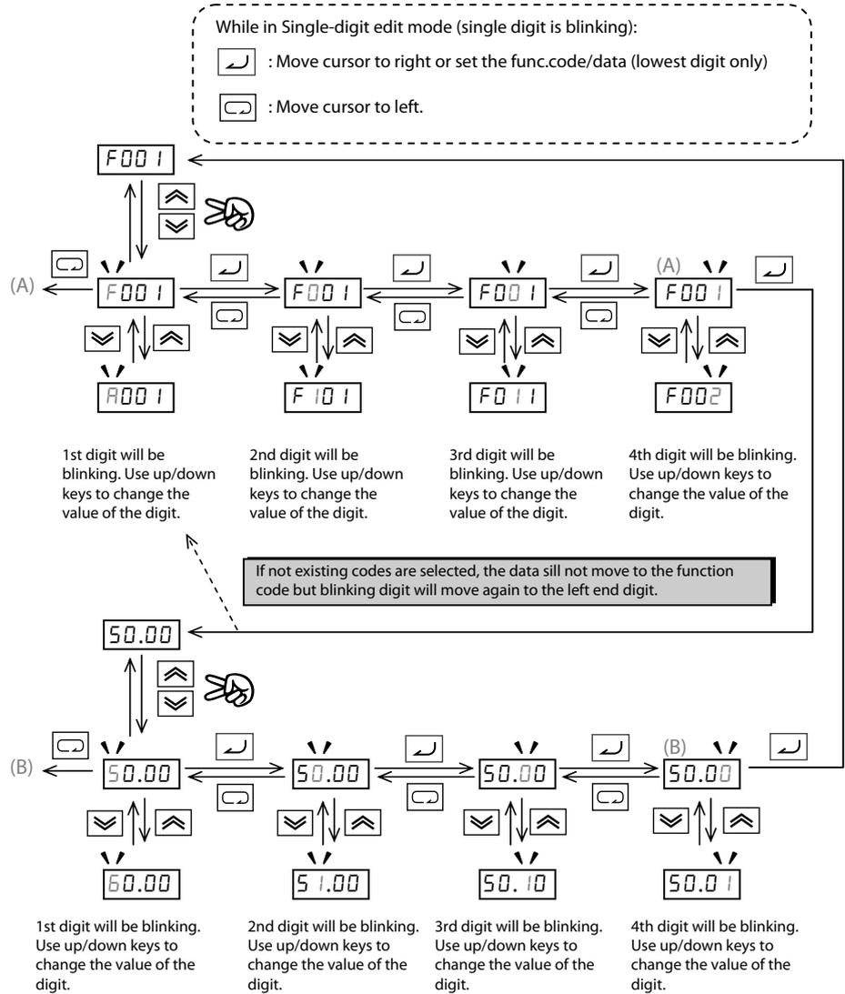
**Note** When pressing with cursor on the highest digit, the cursor will jump to the lowest digit. ((A) and (B) in above figure.)
