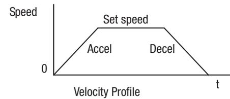
Acceleration and deceleration settings specify the time required to go from a stop to maximum frequency (or vice versa). The resulting slope (speed change divided by time) is the acceleration or deceleration. An increase in output frequency uses the acceleration slope, while a decrease uses the deceleration slope. The accel or decel time a particular speed change depends on the starting and ending frequencies.
