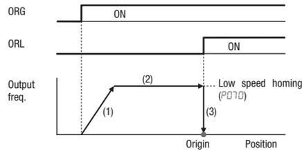
1. The inverter accelerates the motor for the specified ramp time to the low speed homing.
