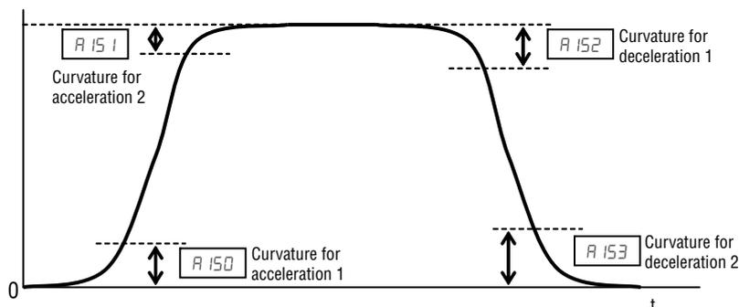
For use of EL-S curve be sure to use select multi-speed as frequency source to avoid nuisance change of frequency during acceleration and deceleration.
