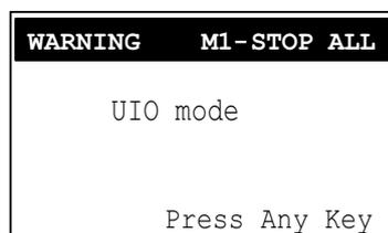
This mode is cancelled by pressing any key, but the WARNING LED and the orange backlight lighting are not cancelled. During "Unprotected Inverter Operation mode", d090 (Warning monitor) displays "UIO". Moreover, the WARNING mode screen displays the following screen:
