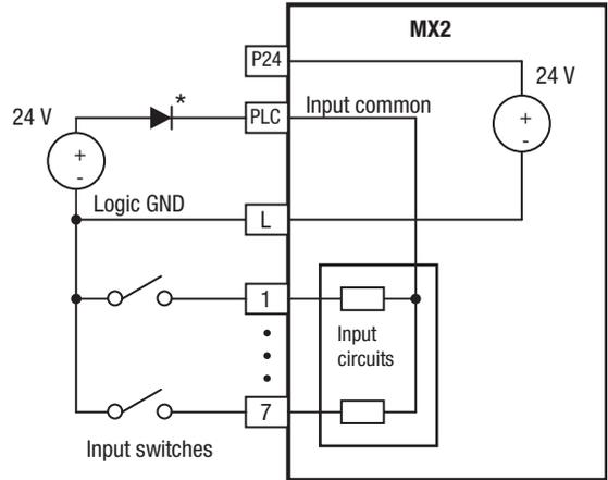
\* Note: If the external power supply to GND is (optionally) connected to [L], then install the above diode.
