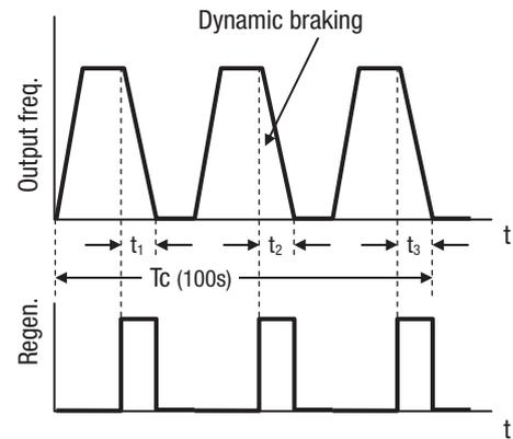
$$b090 \quad T\% = \frac{t_1 + t_2 + t_3}{100 \text{ sec}} \times 100$$
