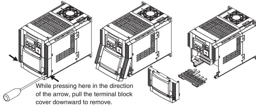
The terminal block cover is secured with one screw at the bottom right for 3.0 kW and smaller models, or with two screws on both sides for 3.7 kW and larger models.
