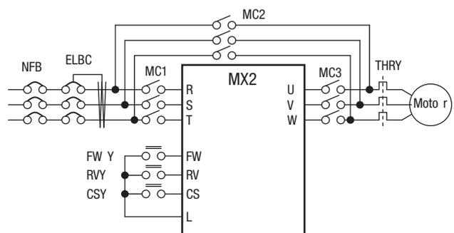
Use weak-current type relays for FWY, RVY, and CSY. The figures below show the sequence and timing of operations for reference.
