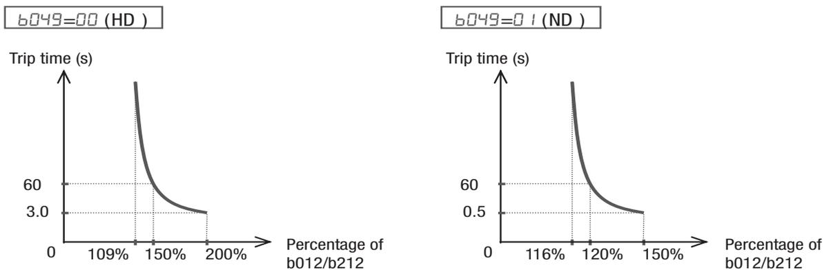
The characteristic curve is unique, but reduction rate depending on frequency is selected in **b013**.
