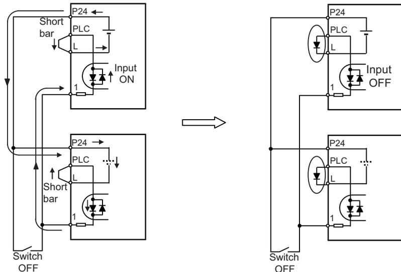
The current loop cause turn the input ON even the switch is off when diode is not inserted.
