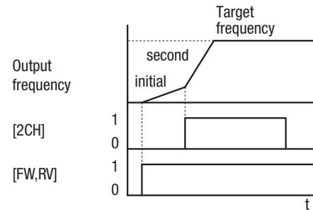
In the graph shown above, the [2CH] becomes active during the initial acceleration. This causes the inverter to switch from using acceleration 1 (*F002*) to acceleration 2 (*A092*).
