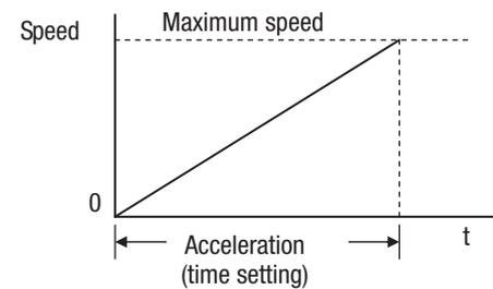
However, the slope is constant, corresponding to the full-scale accel or decel time setting. For example, the full-scale acceleration setting (time) may be 10 seconds - the time required to go from 0 to 60 Hz.
