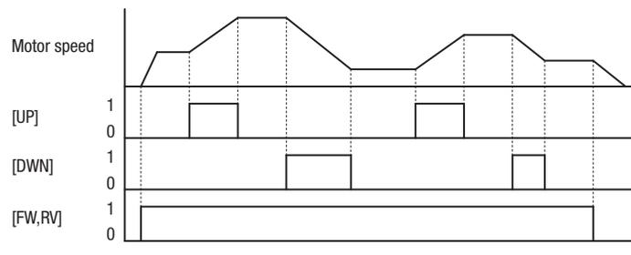
It is possible for the inverter to retain the frequency set from the [UP] and [DWN] terminals through a power loss. Parameter  $C101$  enables/disables the memory. If disabled, the inverter retains the last frequency before an UP/DWN adjustment. Use the [UDC] terminal to clear the memory and return to the original set output frequency.
