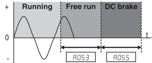
When you set A051 to 01 (Enable during stop), and the RUN command (FW/RV signal) turns OFF, the inverter injects a DC voltage into the motor windings during deceleration below a frequency you can specify (A052).
