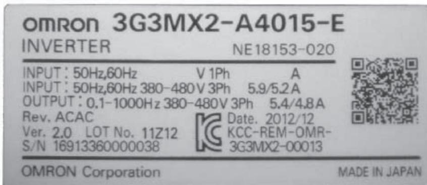
The model number for a specific inverter contains useful information about its operating characteristics. Refer to the model number legend below:
