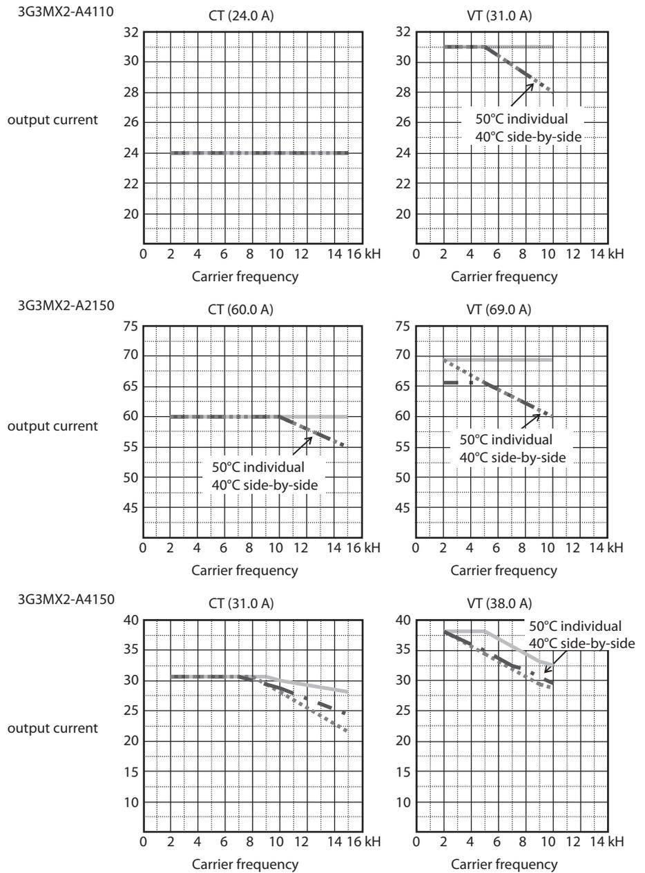
**Ambient Temperature Derating Curves (IP54)**
