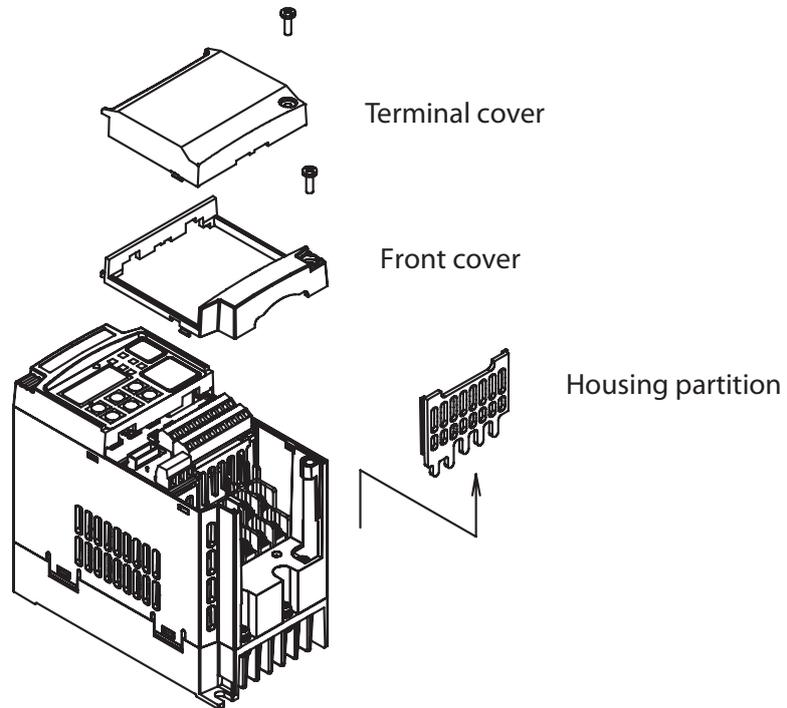
**Note** The housing partition can be removed without removing the front cover in the following models.
