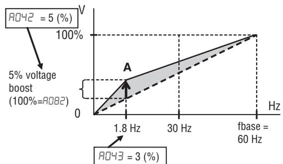
The function attempts to compensate for voltage drop in the motor primary winding in the low speed range.
