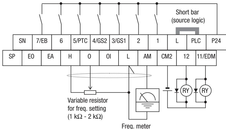
**Note** If relay is connected to intelligent output, install a diode across the relay coil (reverse-biased) in order to suppress the turn-off spike.
