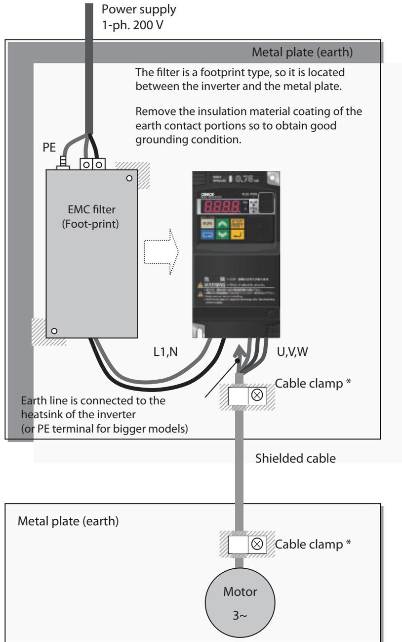
\* Both earth portions of the shielded cable must be connected to the earth point by cable clamps.
