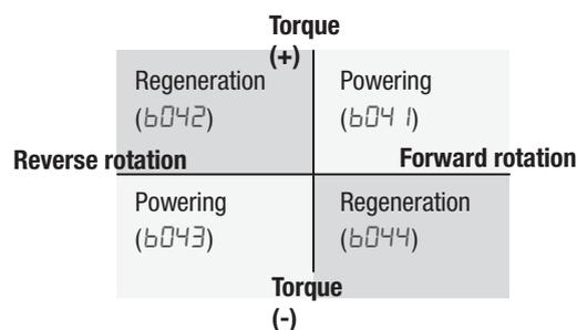
When “01” is specified for the torque limit selection (**b040**), the torque limit 1 to 4 are set as shown to the bottom right. The torque limit 1 to 4 are switched by the torque limit switches 1 and 2 assigned to intelligent input terminals 7 and 8, respectively for example:
