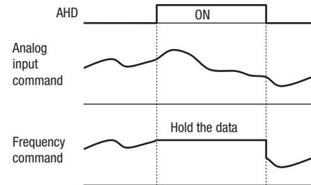
**Note** Set frequency remains when the inverter is switched with SET terminal with AHD on. Turn AHD terminal off to re-hold the set frequency.
