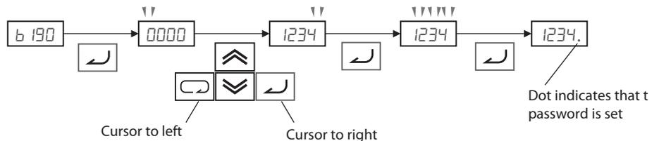
3. Password has been set and locked. Parameter **b037** and/or **b031** cannot be changed.
