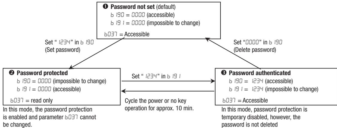
• Function Code Display Restriction Function and Software Lock Function
