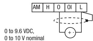
**Current Input** – The current input circuit uses terminals [OI] and [L]. The current comes from a *sourcing* type transmitter; a *sinking* type will not work! This means the current must flow into terminal [OI], and terminal [L] is the return back to the transmitter. The input impedance from [OI] to [L] is 100 Ohms. Attach the cable shield wire only to terminal [L] on the inverter.
