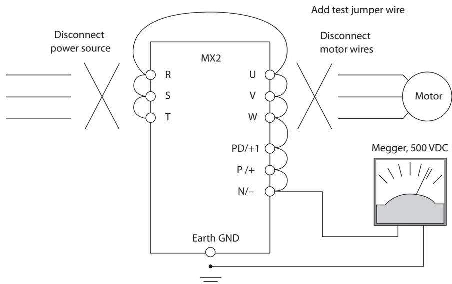
6. After completing the test, disconnect the megger from the inverter.
