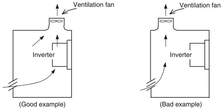
Keep the Inverter away from heating elements (such as a Braking Resistor, reactor, etc.).
