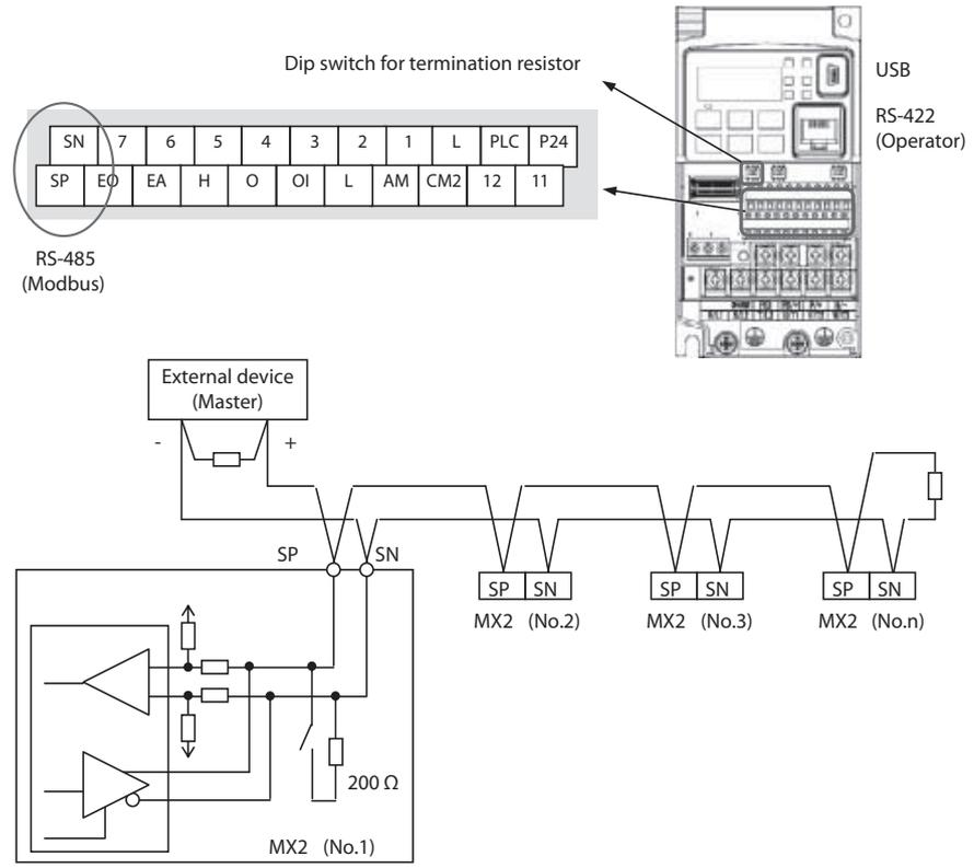
**Terminate Network Wiring** – The RS-485 wiring must be terminated at each physical end to suppress electrical reflections and help decrease transmission errors. MX2 has a built-in 200 resistor activated by a dip switch. Select termination resistors that match the characteristic impedance of the network cable. The diagram above shows a network with the needed termination resistor at each end.
