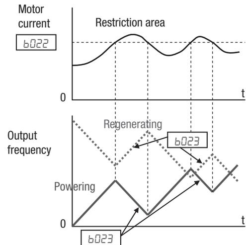
You can specify two types of overload restriction operation by setting functional items b021, b022, b023, and b024, b025, b026 separately. To switch between these two is done by assigning "39 (OLR)" to an intelligent input terminal and make it ON/OFF.
