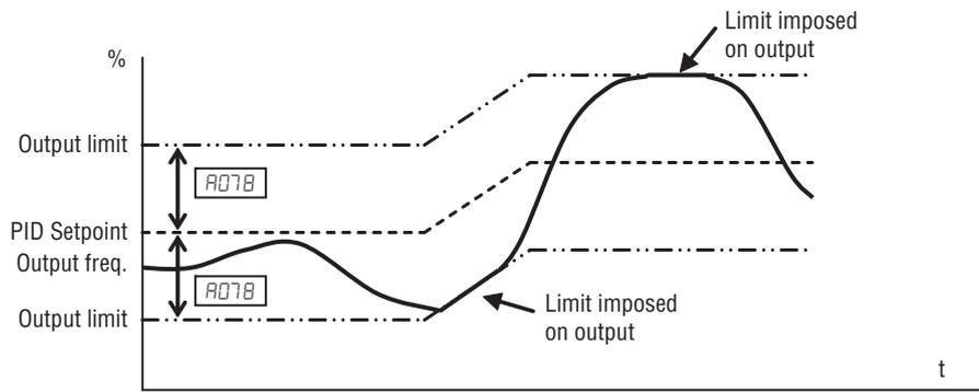
**Deviation (error) Inversion** - In typical heating loops or ventilation loops, an increase in energy into the process results in an *increasing* PV. In this case, the Loop Error = (SP - PV). For cooling loops, an increase in energy into the process results in a *decreasing* PV. In this case, the Loop Error = -(SP - PV). Use **A077** to configure the error term.
