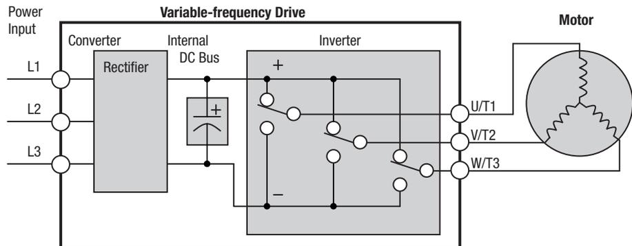
The simplified drawing of the inverter shows three double-throw switches. In Omron inverters, the switches are actually IGBTs (insulated gate bipolar transistors). Using a commutation algorithm, the microprocessor in the drive switches the IGBTs on and off at a very high speed to create the desired output waveforms. The inductance of the motor windings helps smooth out the pulses.
