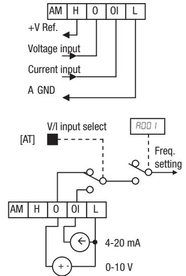
**Note** If no logic input terminal is configured for the [AT] function, then inverter recognizes that [AT]=OFF and MCU recognizes [O]+[OI] as analog input. In case either (O) or (OI) is to be referred, please ground the other.
